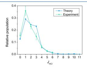
**Figure 2.** Rotational state distribution of the HCl product at 5.5 kcal/ mol collision energy of the  $Cl(^{2}P_{3/2}) + C_{2}H_{6}(v = 0) \rightarrow HCl(v = 0, J_{HCl}) + C_{2}H_{5}$  reaction. The theoretical results, obtained on the present PES, are compared to experimental data taken from ref 8.
